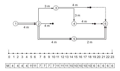
Critical path is marked by double arrow. The dotted lines show the total float of each activity. The requirement of masons for each activity is marked under the activity arrow.
